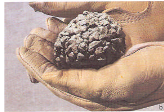
Proper Amount of Water
