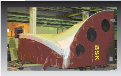
Figure 2 (above). Half-canopy in steel form.
