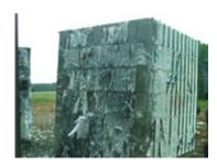
We poured 6 "Reaction Boxes", which are 8 foot cubes with one side open, which were subjected to explosives and live ammunition to see how the insulated concrete walls resist blast force. These tests were conducted at the Quantico Marine Corps Base ranges during a three day period from May 6-8, 2003.
