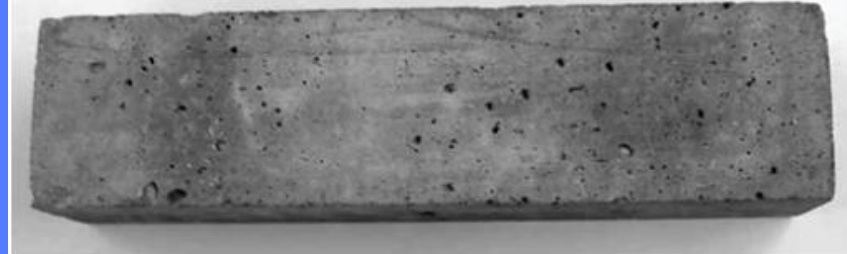
Fig. 5—Specimen subjected to 95 weeks of exposure to 1.06 molal ion concentration solution of CaCl 2 .
