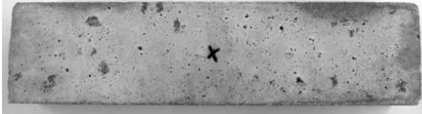
Fig. 4—Specimen subjected to 95 weeks of exposure to 1.06 molal ion concentration solution of NaCl.
