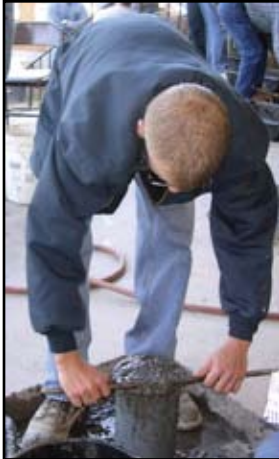
Examination participant leveling out concrete.
