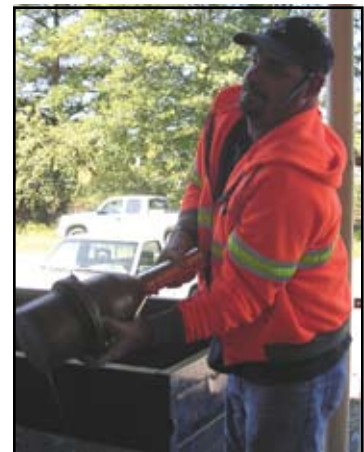
Student performing the tricky task of shaking the volumeter.
