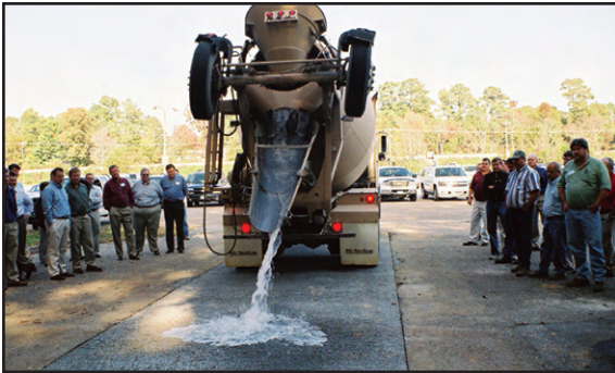
300 gallons of water being dumped on pavement.
