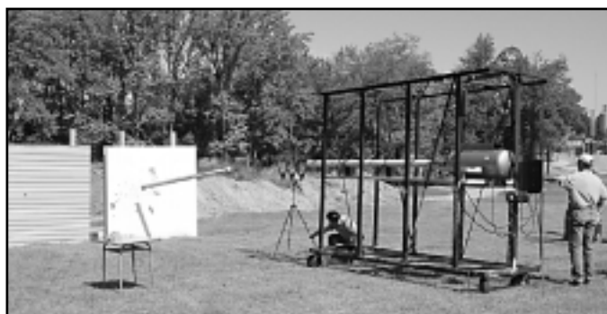
Clemson University air cannon fires at test walls.
