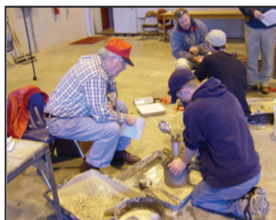
Bill Crummett examines the pressure meter test.
