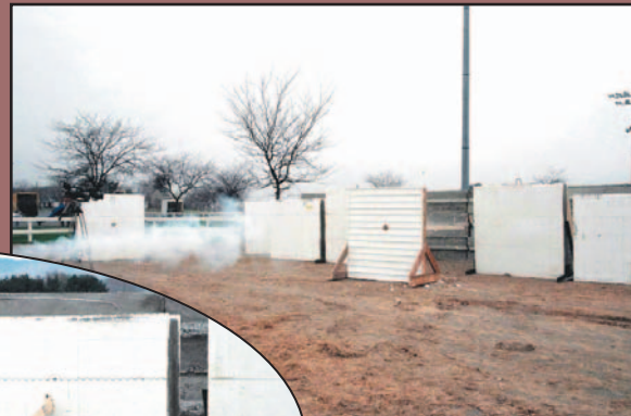
Left: 2x4 timber projectile fails to penetrate concrete-filled ICF wall.
