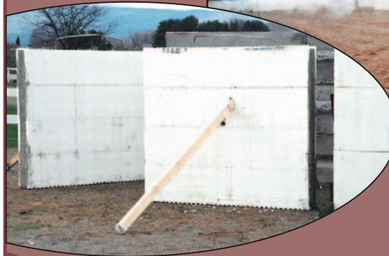
Right: Wind Cannon penetrates 2x6 framed wall with television camera in the background.
